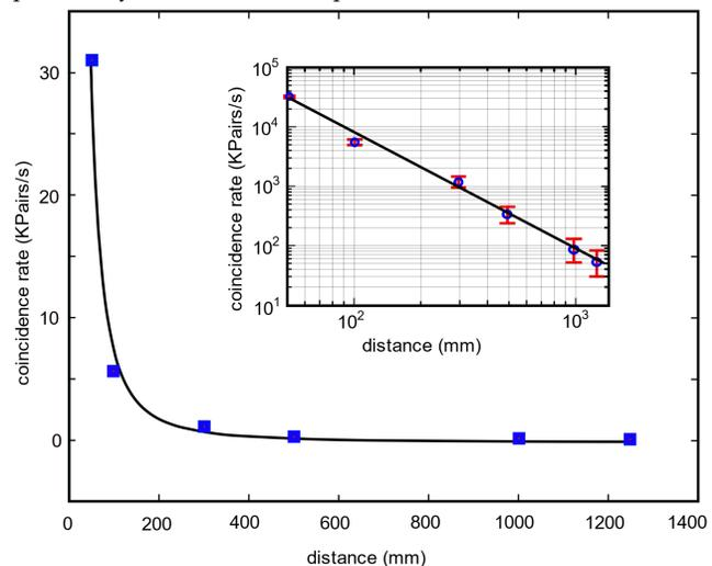
Figure 5: Cross-correlation delay values are converted to distance. The solid black line shows the theoretical fit to the experimental data. The inset shows the logarithmic scale for the ease of reading.
