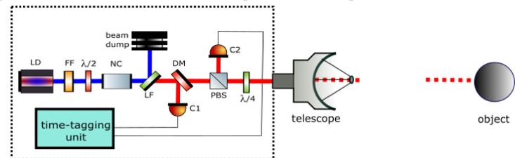
Figure 4: Schematic of the experimental setup to test the proof-of-principle quantum radar concept
