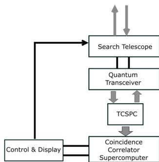
Figure 1: Block diagram of quantum radar design.
